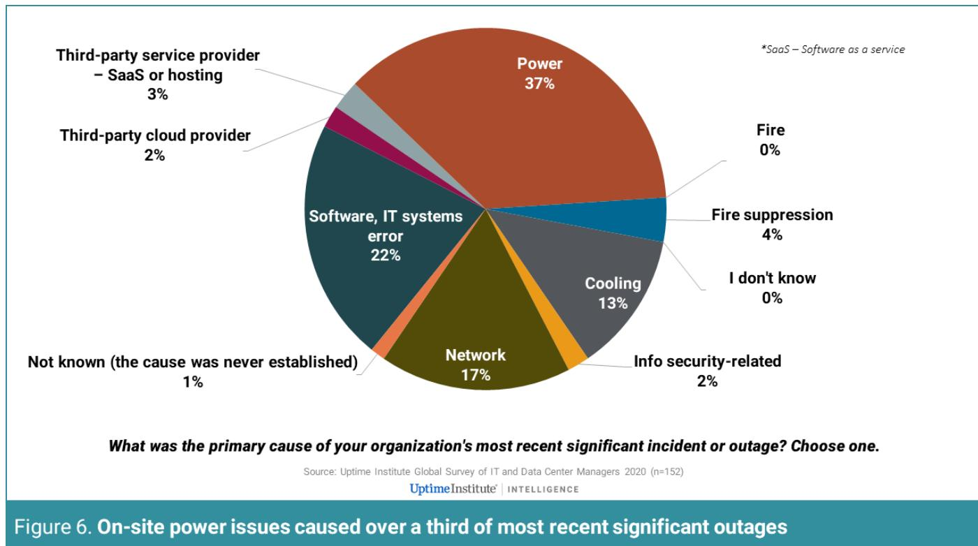
Figure 6. On-site power issues caused over a third of most recent significant outages
